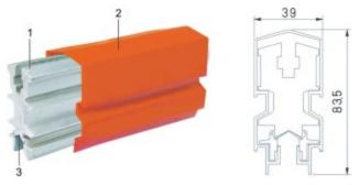
The conductor (1) is in aluminum material, with vertical and horizontal direction stiffness, and large surface area, guaranteeing fully heat dissipation. It has stainless steel conductor ③ as the durable surface. The sheath 2 can meet safety standard in IP23, and it's shape is waterproof and dust proof.
