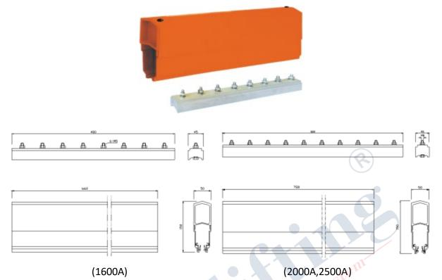
The joint plate is in aluminum material, using 8 or 10 bolts according to the conductor bar's specification, so it can ensure each conductor bar's linearity and conductive continuity.
