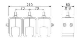
The Max. distance between hanger clamps is 3m.
