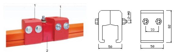
The fixation clamps  $\bigcirc$  are usually used in pairs, installed on both sides of the hanger clamp  $\bigcirc$ , which is in the middle of the system or between the two expansion sections.
