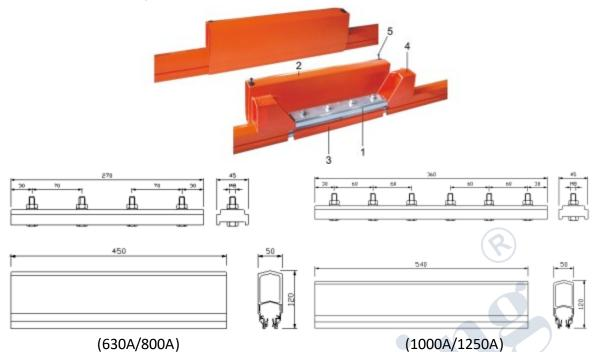
The joint plate ① is in aluminum material, using 4 or 6 bolts according to the conductor bar's specification, so it can ensure each conductor bar's linearity and conductive continuity.
