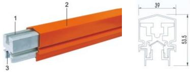
The conductor ① is in aluminum material, with vertical and horizontal direction stiffness, and large surface area, guaranteeing fully heat dissipation. It has stainless steel conductor ③ as the durable surface.
