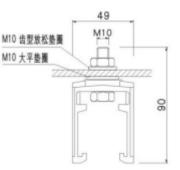
The Max. distance between hanger clamps is 3m.
