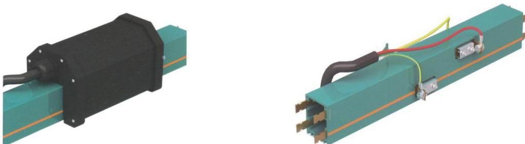
The line feeding is provided with 0.5m conductor rail. Other lengths are available, but should not exceed 4 meters. 56ZG/500-4/50A, means 4 poles and 50 Amp conductor rail.
