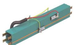
The line feeding is provided with 0.5m conductor rail. Other lengths are available, but should not exceed 4 meters. 56ZG/500-4/50A, means 4 poles and 50 Amp conductor rail.
