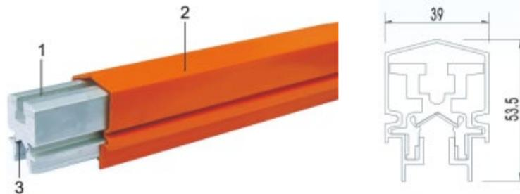
The conductor① is in aluminum material, with vertical and horizontal direction stiffness, and large surface area, guaranteeing fully heat dissipation. It has stainless steel conductor③ as the durable surface.
