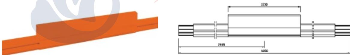
The expansion section is equipped with key sliding part. The overlap of copper strips can be used as sliding wire's contact surface, so as to ensure the continuity of the conductive. Copper rod slides in the plastic conductive bearing, which plays a machinery guiding role. At both ends of the connector sheath, there are end cover and fixed plastic bolt. The maximum Gap is 200mm.
