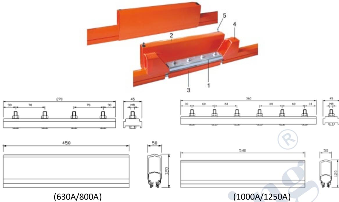
The joint plate ① is in aluminum material, using 4 or 6 bolts according to the conductor bar's specification, so it can ensure each conductor bar's linearity and conductive continuity.
