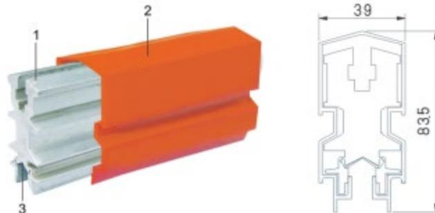
The conductor① is in aluminum material, with vertical and horizontal direction stiffness, and large surface area, guaranteeing fully heat dissipation. It has stainless steel conductor③ as the durable surface. The sheath ② can meet safety standard in IP23, and it's shape is waterproof and dust proof.
