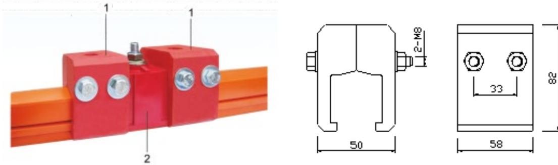
The fixation clamps ① are usually used in pairs, installed on both sides of the hanger clamp ②, which is in the middle of the system or between the two expansion sections.
