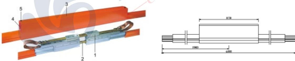
The expansion section is equipped with key sliding part①. The overlap of copper strips② can be used as sliding wire's contact surface, so as to ensure the continuity of the conductive. Copper rod slides in the plastic conductive bearing, which plays a machinery guiding role. At both ends③ of the connector sheath, there are end cover④, and fixed plastic bolt⑤. The maximum Gap is 200mm.
